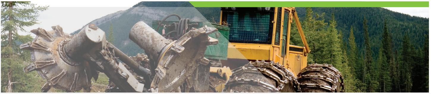
Other Pierce products include attachments for the logging industry, such as delimers that process a cut log while a computer simultaneously measures the diameter of the log, delivering cutting instructions based on the customer's requirements. Pierce Pacific also manufactures grapples, log loaders, high speed saws, and scrap machines that move bulk materials onto or from barges. The machines characterize Pierce Pacific equipment which does more with less manpower.
